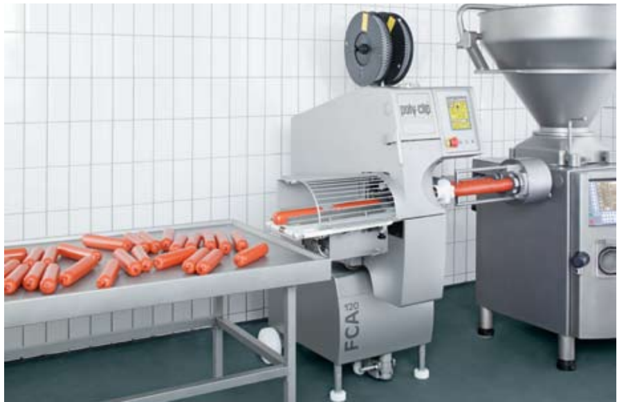
FCA 120 - the specialist machine for high speed production of calibres up to 120 mm
