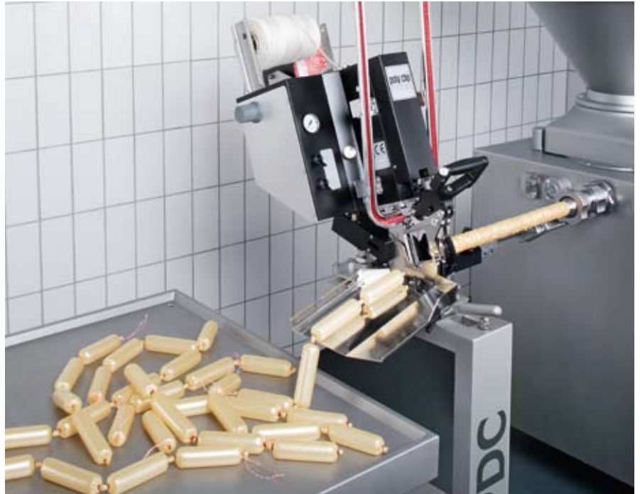
Products with diameters up to 80 mm in diameter can be produced quickly and safely with the PDC 600
