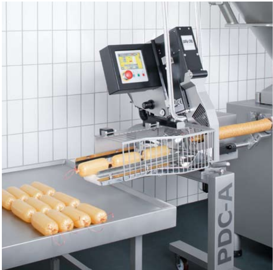
The PDC-A automatic double-clipper reliably closes all artificial, fibrous, collagen and natural casings
